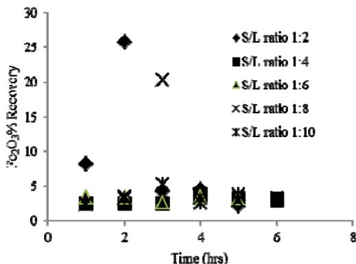
Fig. 5. Effect of solid to liquid ratio on Fe<sub>2</sub>O<sub>3</sub> recovery
