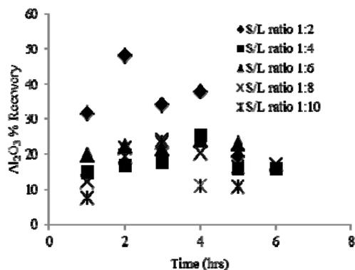
Fig. 4. Effect of solid to liquid ratio on Al<sub>2</sub>O<sub>3</sub> recovery
