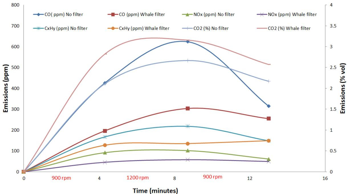
**Fig. 4.** Average exhaust emissions for Bus at various engine speeds before and after Whale filter installation.
