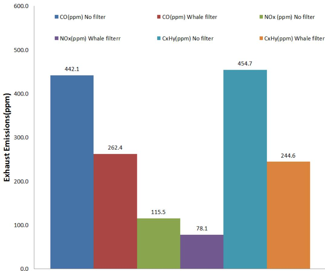
Fig. 9. Average exhaust emissions for John Deere 7800 Tractor before and after Whale filter installation.
