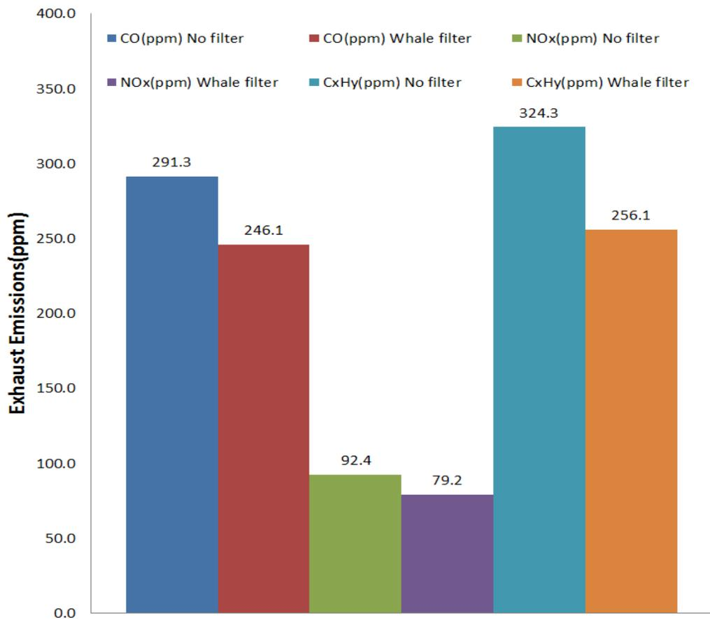
Fig. 7. Average exhaust emissions for BELL 315SJ TLB before and after Whale filter installation.
