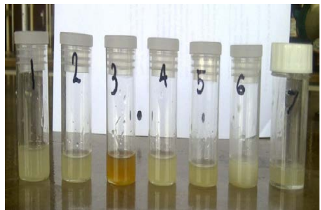
Fig. 7 Oil colour variation with microwave setting
