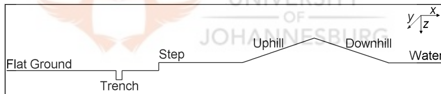
Figure 3.2: Terrain model developed for testing.
