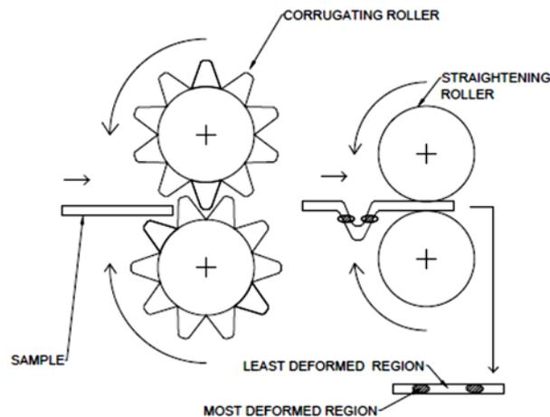
**Figure1. Corrugated and straightened sample in a continuous process tool**
