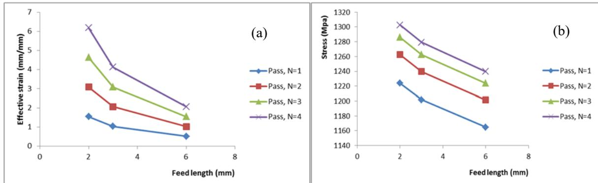
**Figure 3. (a) Effective strain vs feed length (b) Tensile true stress vs feed length.**
