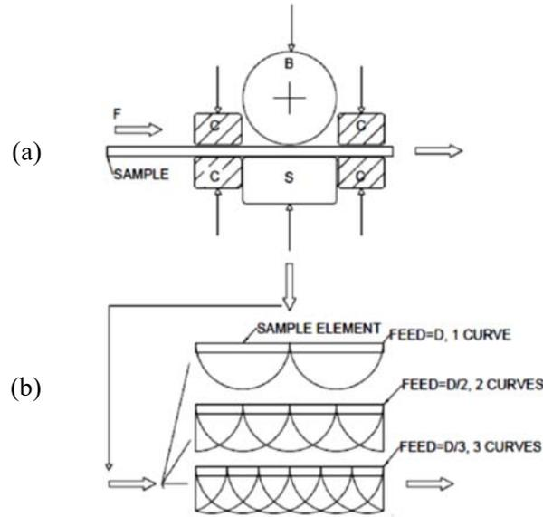
**Figure 2. (a) Principle of CBS (b) Feed length and respective bending curves in CBS**
