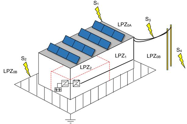
Figure 1: Lightning protection zones based on point of strike
