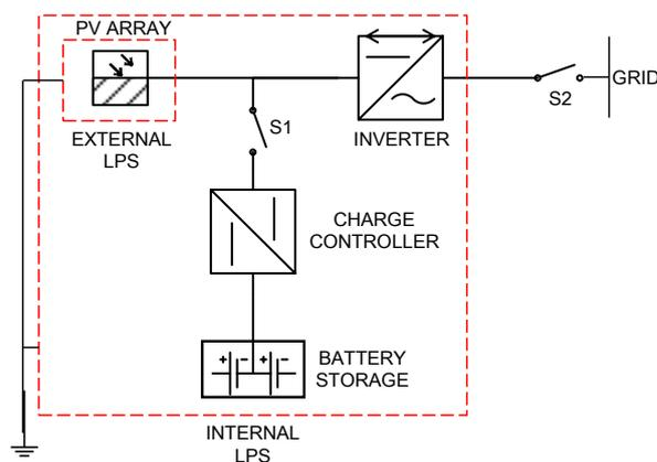
Figure 3: External and internal LPS for PV components
