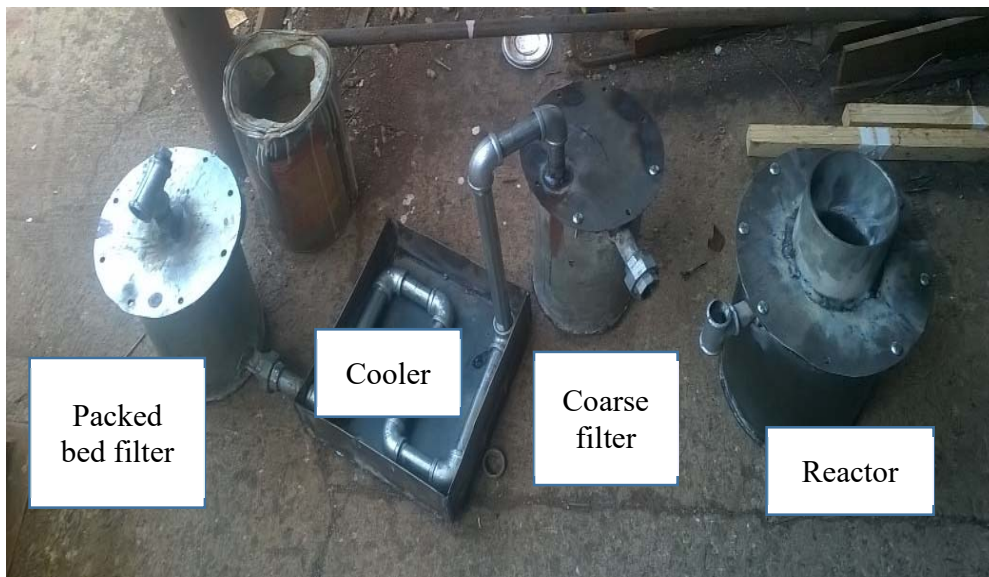
Figure 8 Fabricated Sub-Assemblies of actual prototype layout
