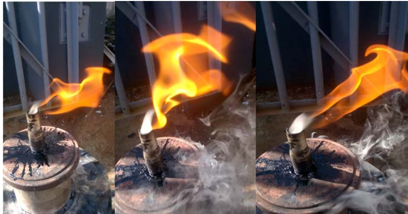
Figure 9 Syngas burning (University of Zimbabwe Mechanical Engineering Workshop)
