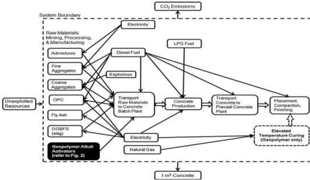
Fig. 1. CO2 emissions diagram in producing 1m<sup>3</sup> of concrete [14]
