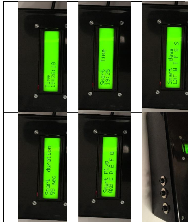
Fig. 5. Complete central control unit with user interface, and the different menus.
