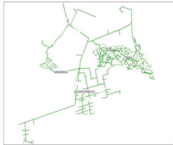
Fig. 2: MV feeder network for Taunus substation [25]
