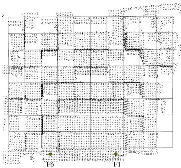
Fig. 8. Plan view of the combined and filtered point clouds
