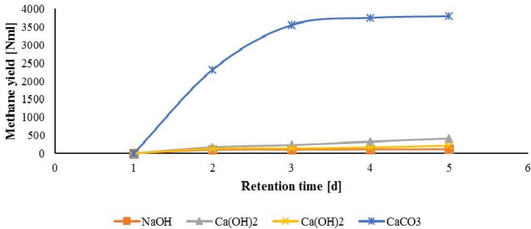
Fig. 2: Cumulative methane yield from the different digesters
