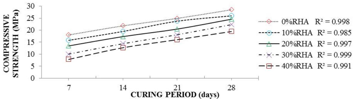
Fig. 6: Compressive strength of respective concrete samples
