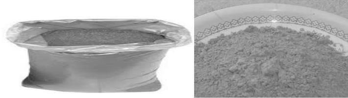
Fig. 3: Controlled incinerated RHA
