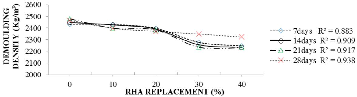
Fig. 5: Effect of RHA replacements on concrete density
