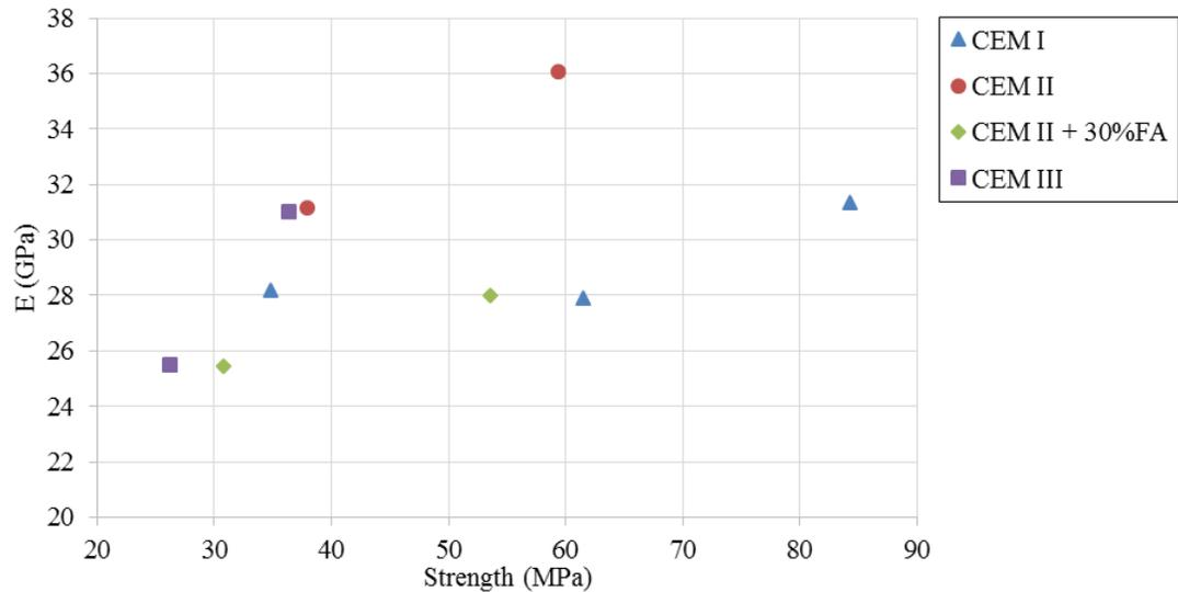
**Fig. 4.** Specimen results containing andesite cured for 7 days
