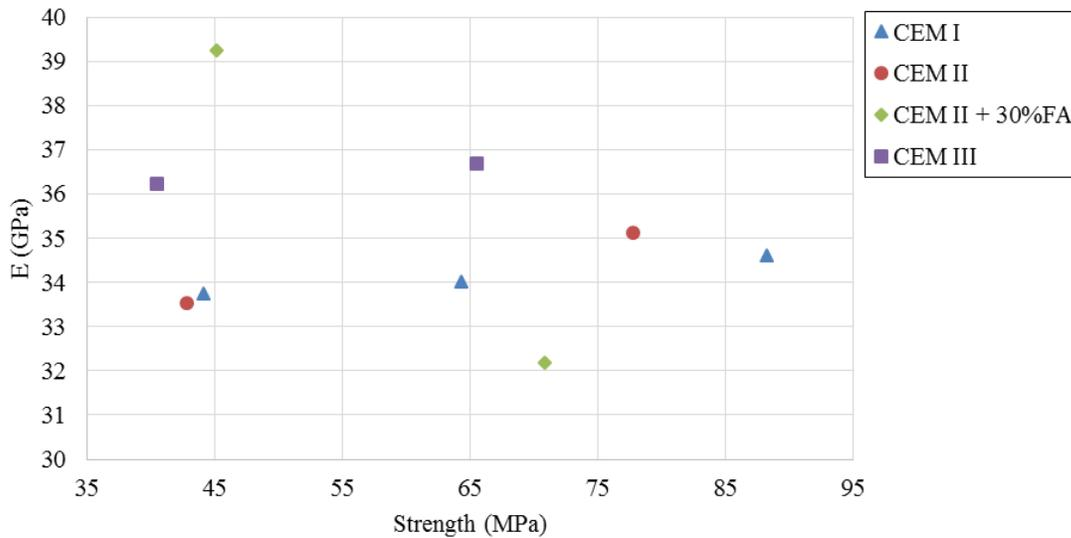
**Fig. 14.** Specimen results containing quartzite cured for 56 days
