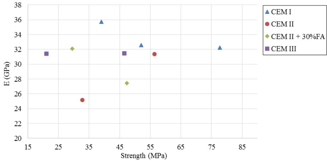
**Fig. 6.** Specimen results containing quartzite cured for 7 days
