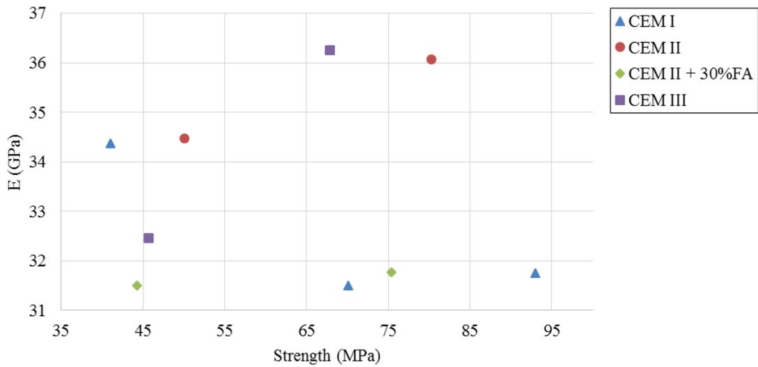
**Fig. 12.** Specimen results containing andesite cured for 56 days
