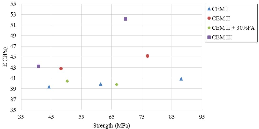
**Fig. 13.** Specimen results containing dolomite cured for 56 days
