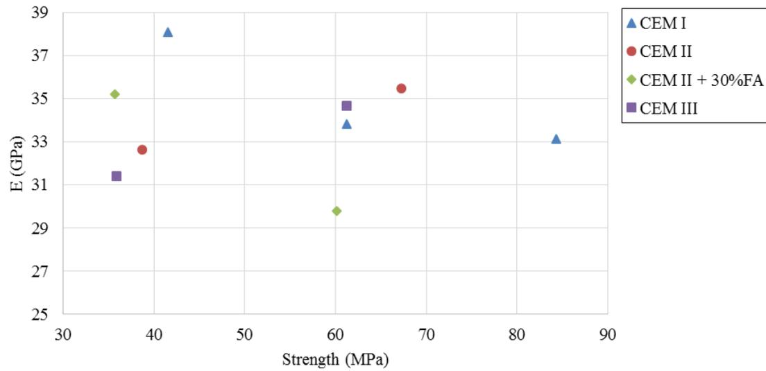
**Fig. 10.** Specimen results containing quartzite cured for 28 days
