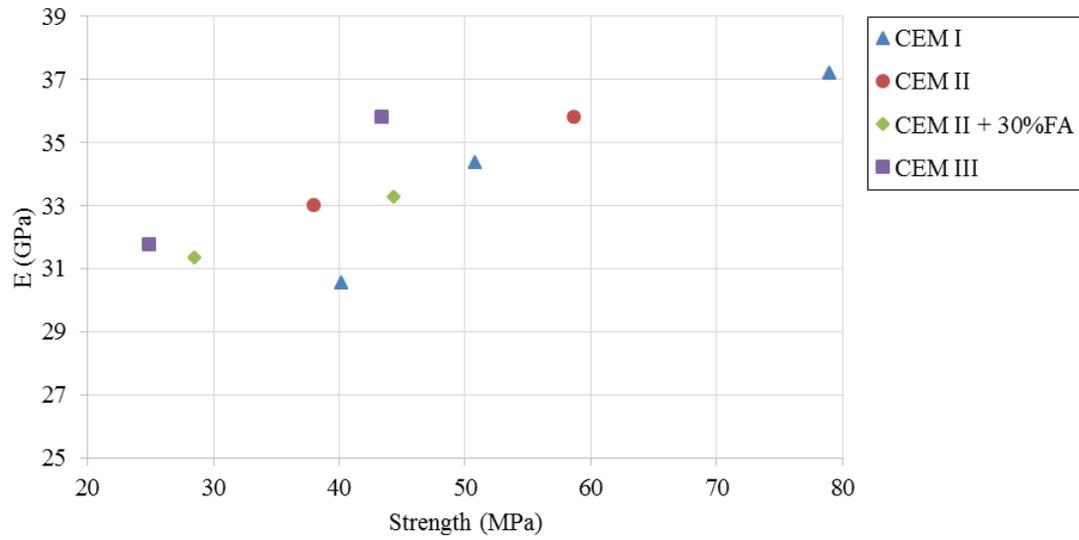
**Fig. 5.** Specimen results containing dolomite cured for 7 days
