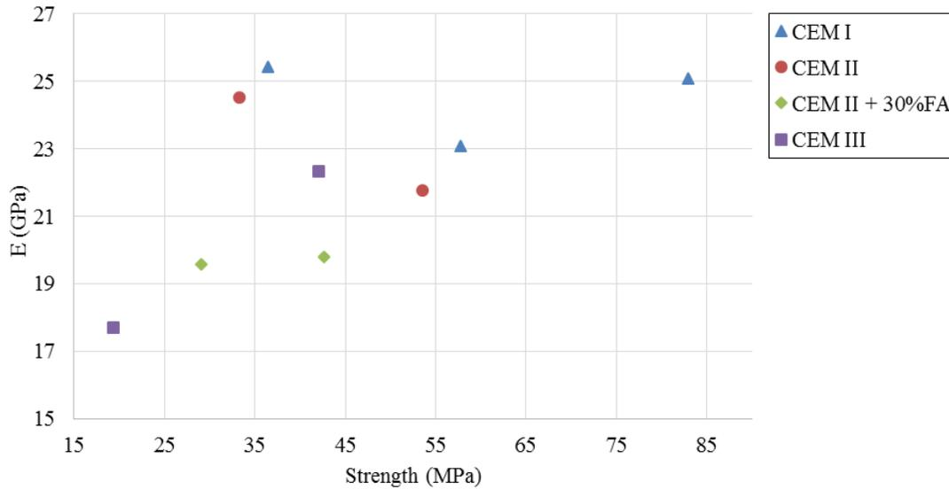
**Fig. 7.** Specimen results containing granite cured for 7 days
