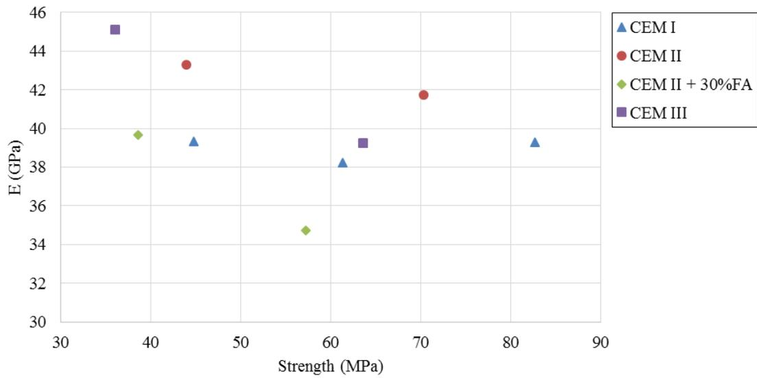
**Fig. 9.** Specimen results containing dolomite cured for 28 days
