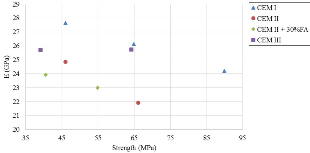
**Fig. 11.** Specimen results containing granite cured for 28 days
