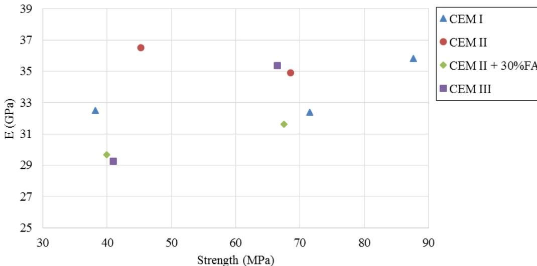
**Fig. 8.** Specimen results containing andesite cured for 28 days
