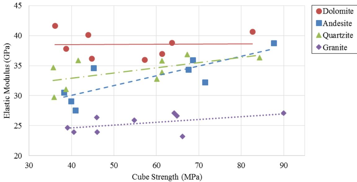
**Fig. 2.** Effect of aggregate type on 28 day cured concrete
