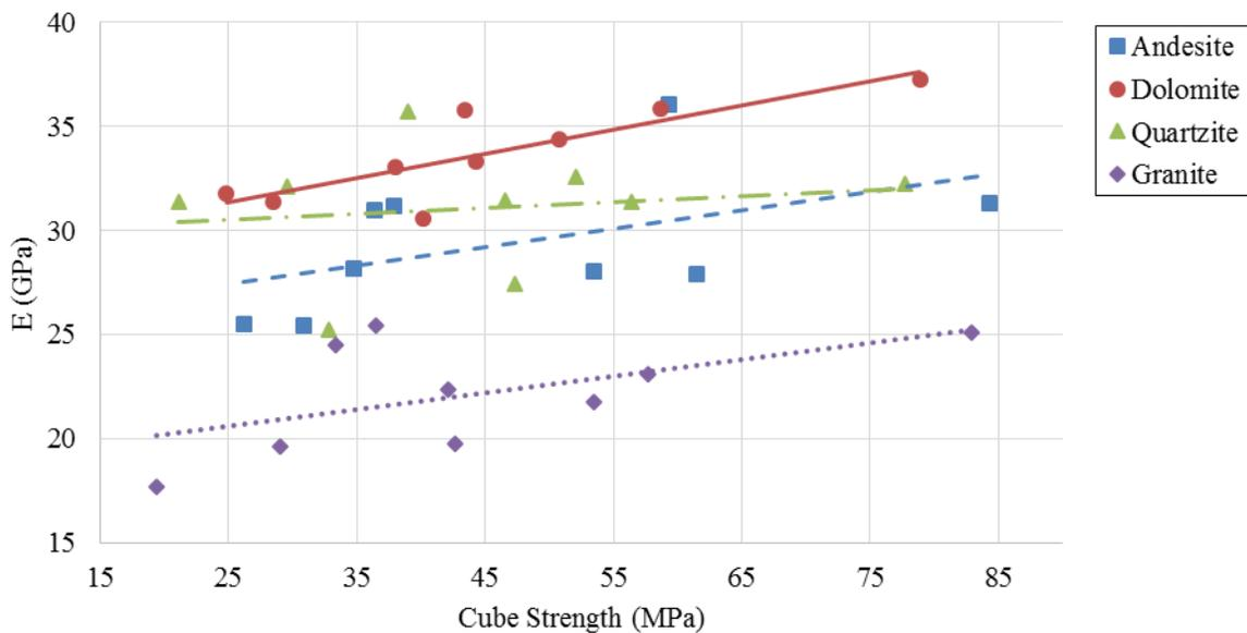
**Fig. 4.** Effect of aggregate type on 7 day cured concrete normalized according to the mean percentage content of aggregate
