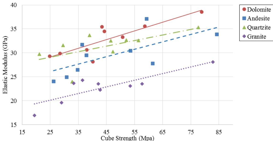
**Fig. 1.** Effect of aggregate type on 7 day cured concrete
