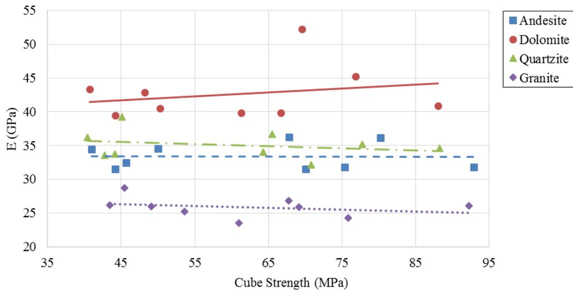
**Fig. 6.** Effect of aggregate type on 56 day cured concrete normalized according to the mean percentage content of aggregate
