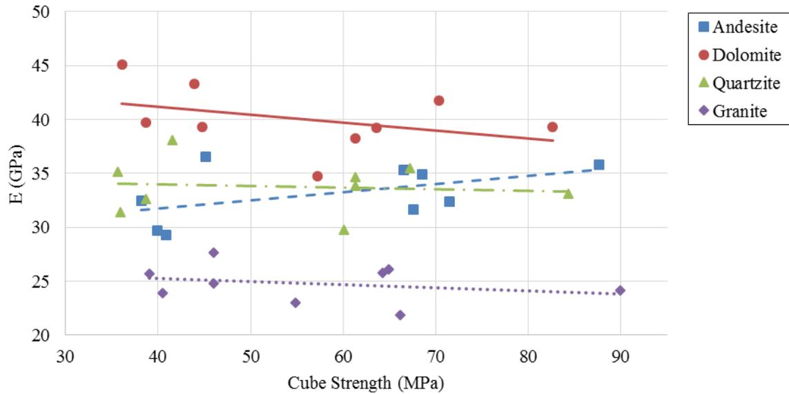
**Fig. 5.** Effect of aggregate type on 28 day cured concrete normalized according to the mean percentage content of aggregate
