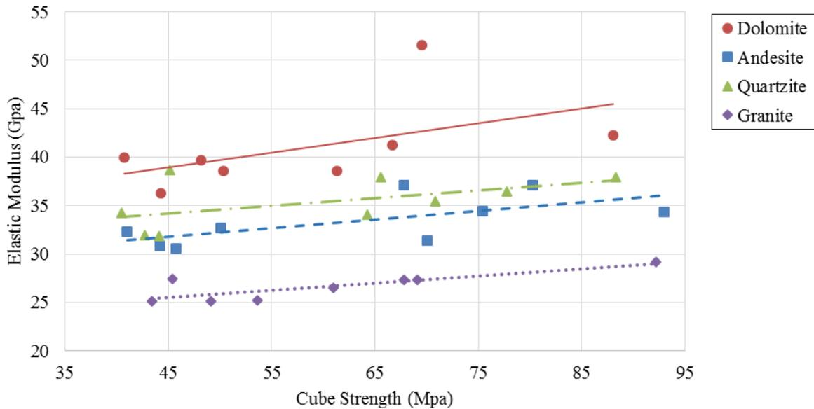
**Fig. 3.** Effect of aggregate type on 56 day cured concrete
