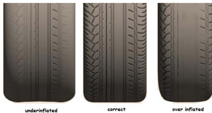
Figure 3. How tyres look like in different cases
