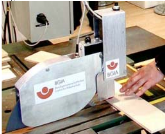
Figure 6. Finger and hand protection on Panel Saws (Dietmar Reinert, 2009)
