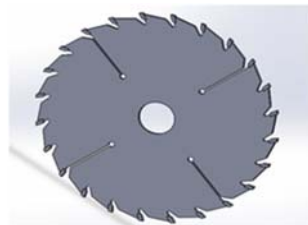
Figure 8. A 350 mm diameter cross-cut saw blade
