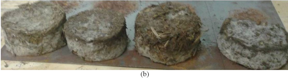
Figure 4: Loose biomass briquettes produced (a) with cow dung binder (b) with cactus binder
