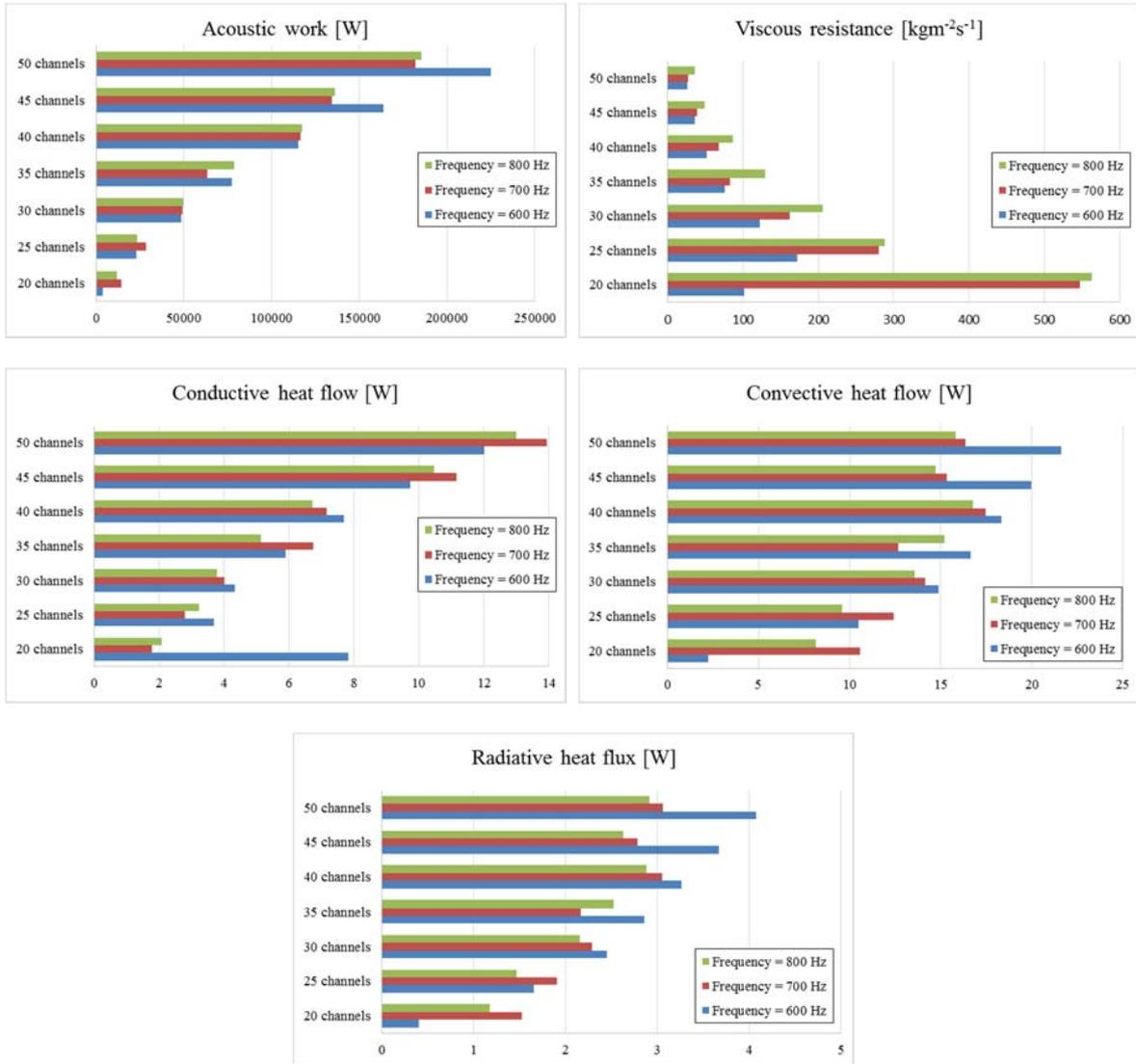
Figure 5: Acoustic work, viscous resistance and heat flows
