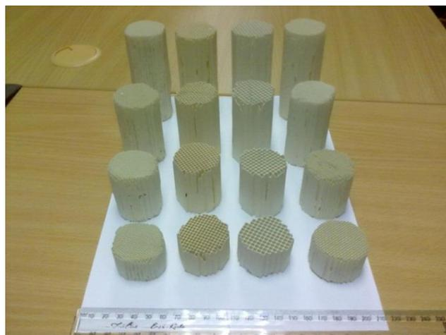
Fig.3: Stack samples used in the experiments/ TAR
