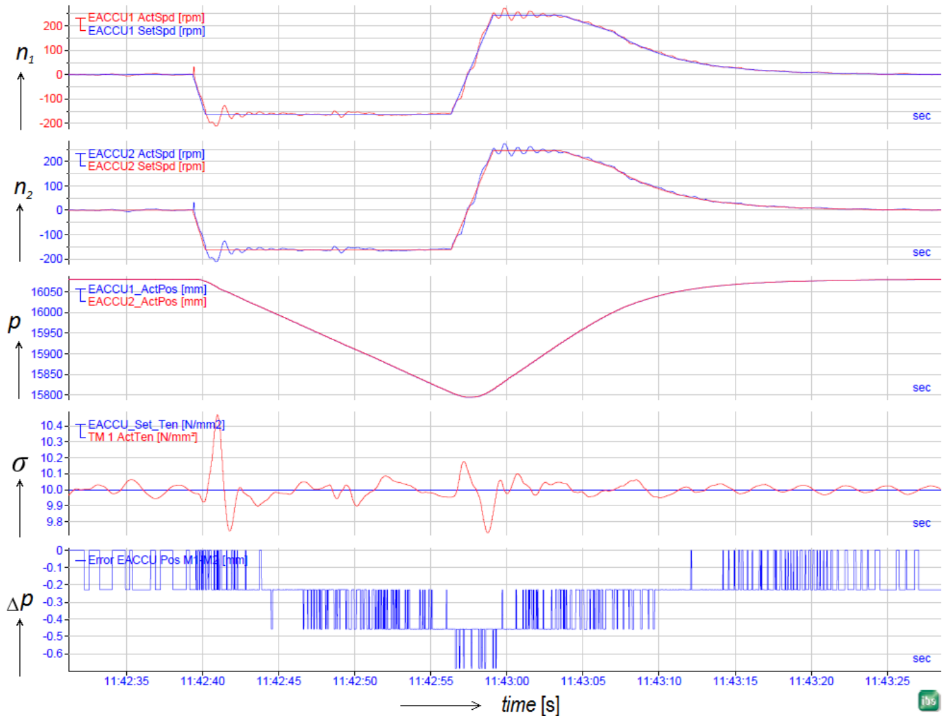
Figure 9. Time courses of the variables at the accumulator filling up and discharging
