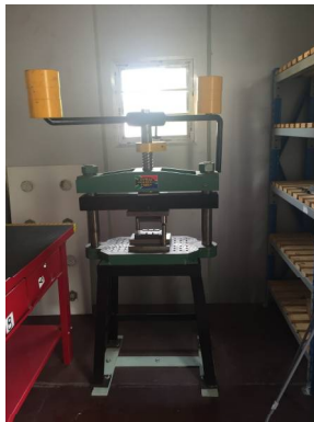
Figure 5: Off grid manually operated 10 ton bending press
