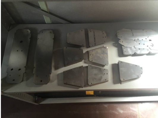
Figure 2: Laser blanked and drilled components designed for community factory manufacture
