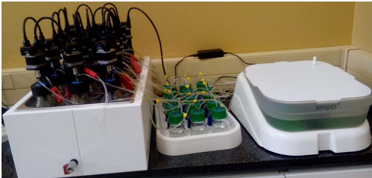
Fig. 1: Bioprocess AMPTS II experimental setup for BMP analysis
