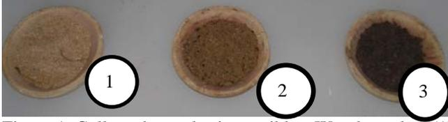
Figure 1. Collected samples in crucibles; Wood sawdust (1), Animal crushed bones (2), Horse dung (3).
