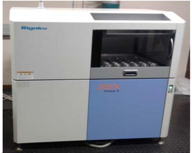
Figure 2: XRF analyzing device (Rigaku ZSX Primus II)
