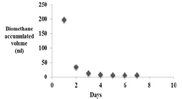
Fig. 4: Biomethane Production from Food waste and cow dung co-digestion (2<sup>nd</sup> Co-digestion).
