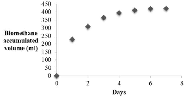
Fig. 3: Biomethane accumulated volume from Cow, pig and grass co-digestion (1<sup>st</sup> co-digestion).
