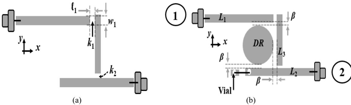
Figure 2: The proposed design design, (a) The feed arrangement, (b) The geometry.
