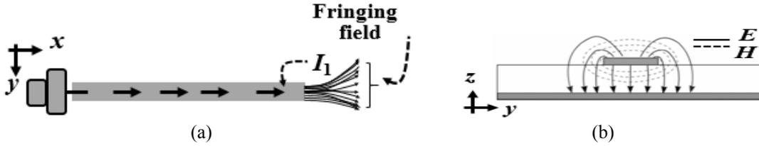
Figure 1: Current effect on microstrip line. (a) Open-ended line, (b) EM field of open-ended line at  $xy$ -plane
