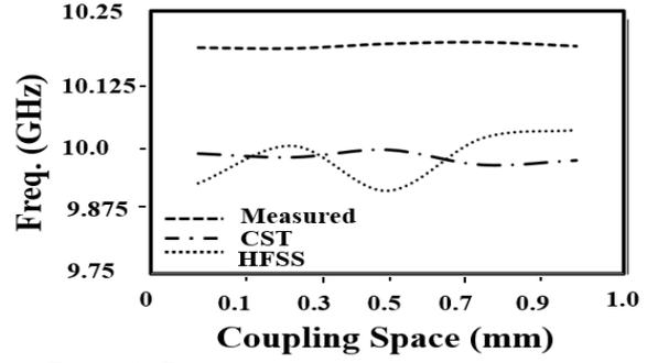
Figure 1: Resonance frequency vs. coupling space.
