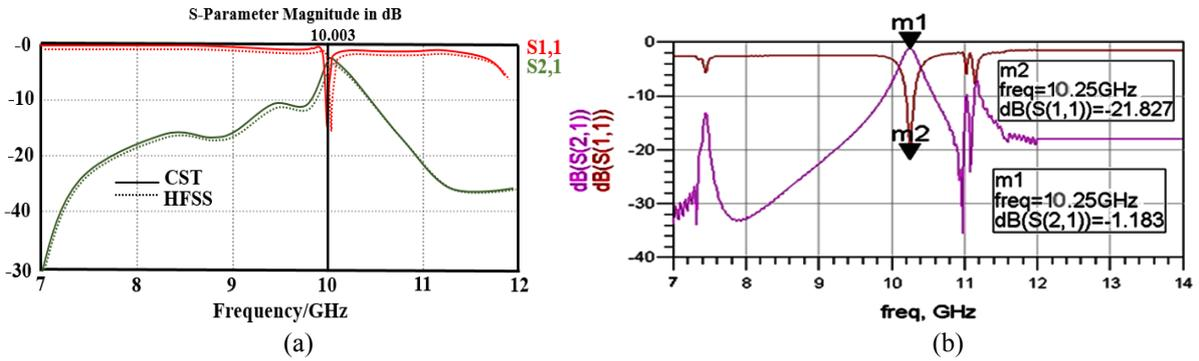
Figure 3: Optimized S-parameter results of the proposed design. (a) Simulation, (b) Measured
