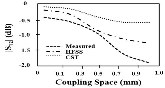
Figure 2: Insertion loss vs. coupling space.
