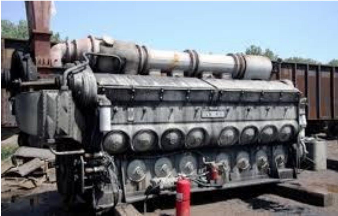
Figure 2: Engine of diesel locomotive (39 200 class) (Transnet, 2014)
