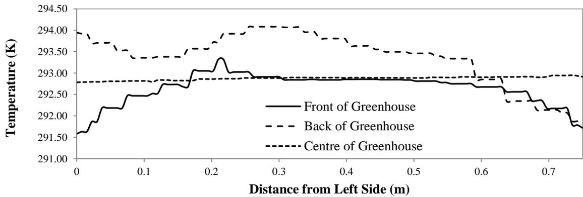
**Figure 10:** Temperature distribution in three planes (front, middle, back) for  $Ra = 4.27 \times 10^8$
