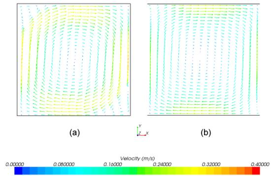
**Figure 3:** Vector plot comparison for (a) Two-dimensional case (b) Three-dimensional case ( $z/H=0.5$ )
