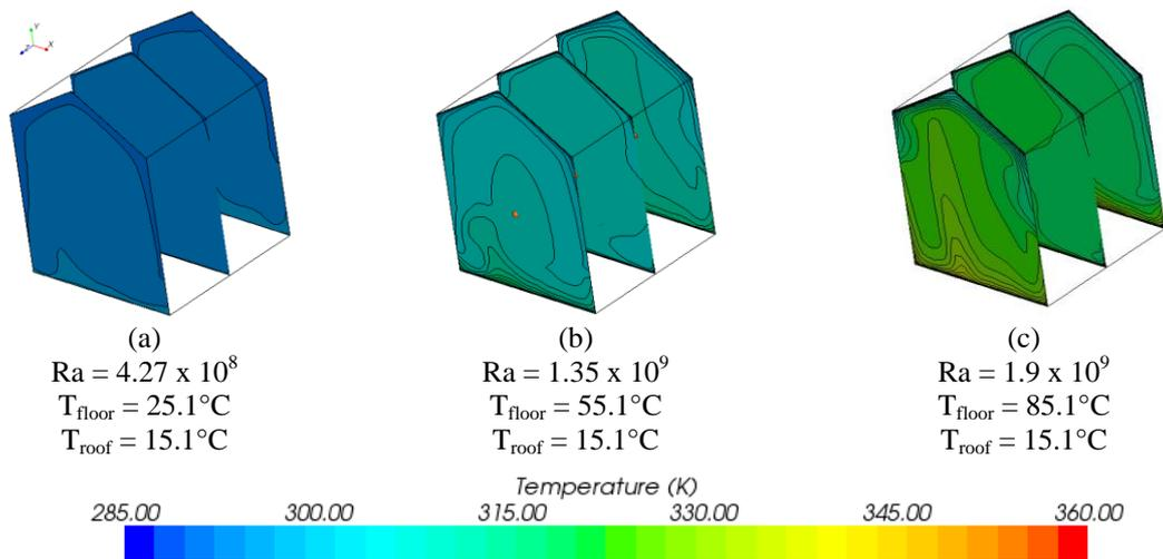
**Figure 9:** Temperature Distribution in three planes (30 Degree Roof Angle)
