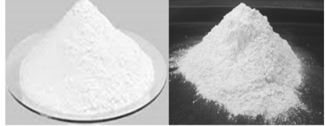
Fig. 2. Pictures showing the fine state of glass activated plastic (GAP) industrial waste powder
