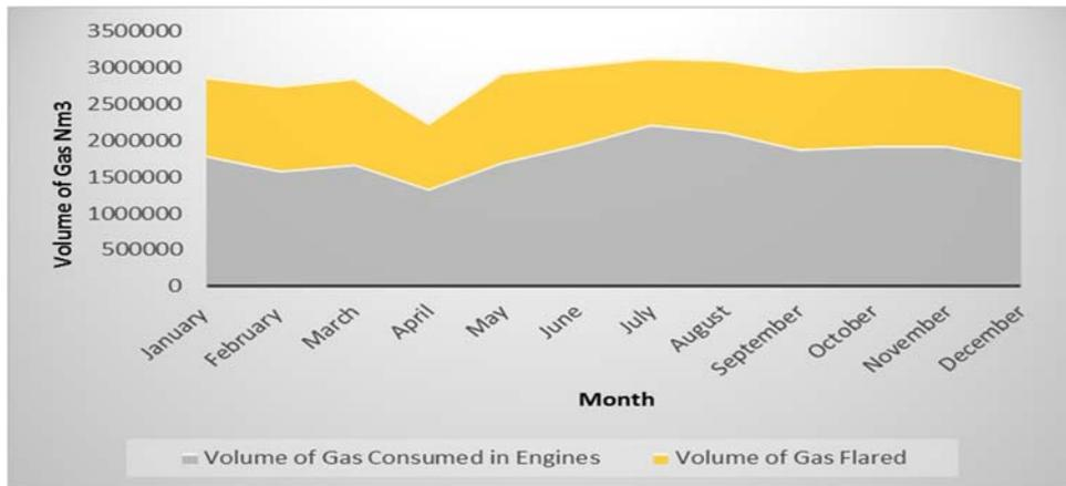
**Figure 4 : Combusted and Flared Gas at Bisasar Road Landfill Site in 2012**
