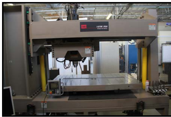
Figure 2: I-STIR friction stir welding machine
