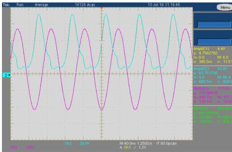
Figure 15. Output voltage (pink) and drain-source voltage (blue)
