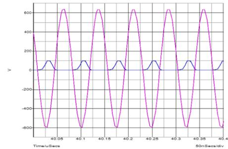
Figure 11 Drain-source voltage (blue) and output voltage (pink)
