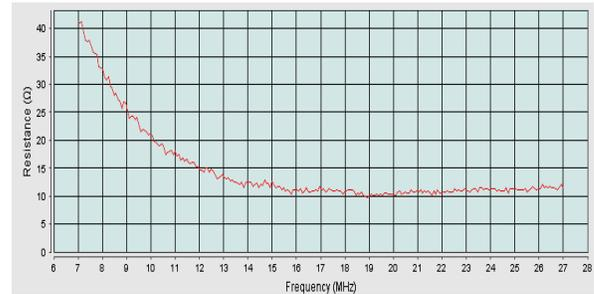
Figure 2. Equivalent series resistance versus frequency
