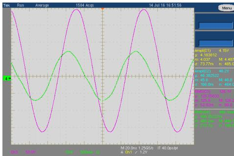
Figure 16 Output parameters: voltage (pink) and current (green)
