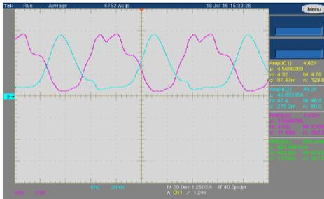
Figure 14. Switch parameters: gate (pink) drain-source voltage (blue)
