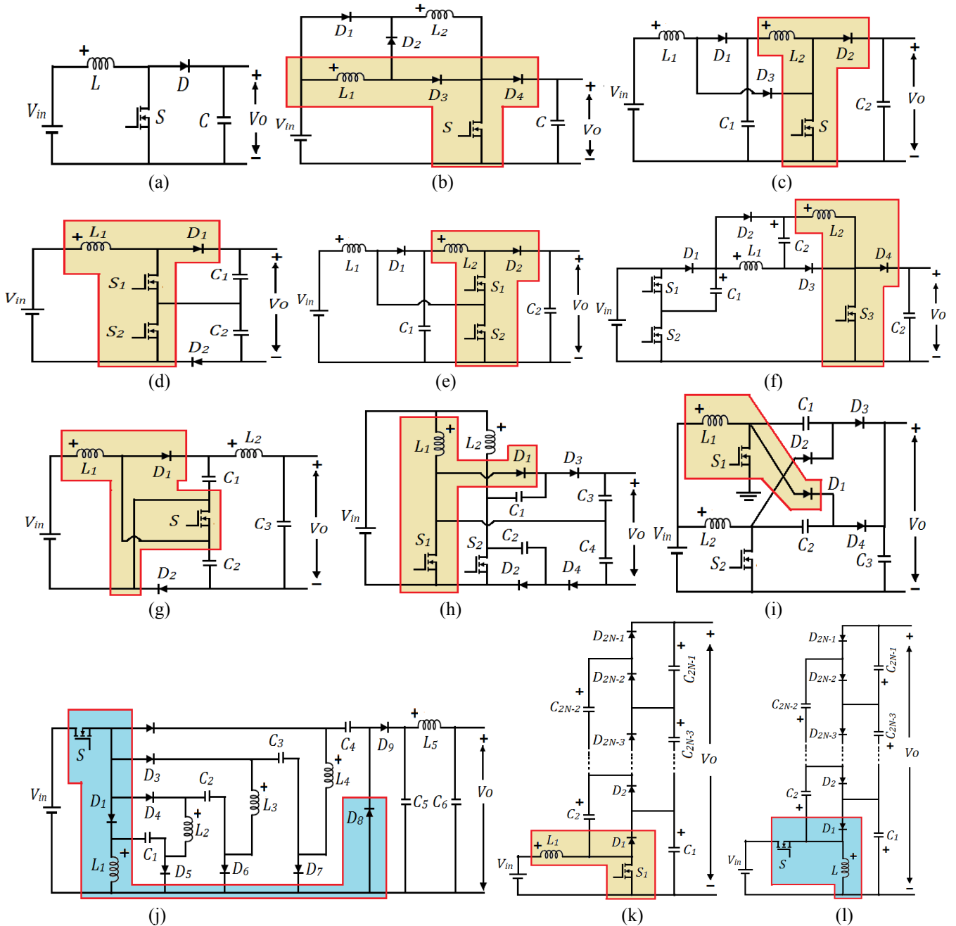
Fig.1(a) Conventional Boost Converter; (b) Switched Inductor (SI) Boost Converter[2]; (c) Single switch Quadratic Boost Converter (QBC) [2],[4] (d) Conventional Three Level Boost Converter [2],[6]; (e) Quadratic Three Level Boost Converter [5]; (f) Converters using bootstrap capacitors and boost inductors; (g) Switched Capacitor Based Boost Converter [7]; (h) Two-phase quadrupled interleaved boost converter [8]; (i) High-voltage gain two-phase interleaved boost converter using one VMC[9]; (j) Extra high voltage (HV) DC-DC converter [10]-[13]; (k) Nx Multilevel Boost Converter (MBC) [14]; (l) inverting Nx Multilevel BuckBoost Converter (MBBC) [14].
