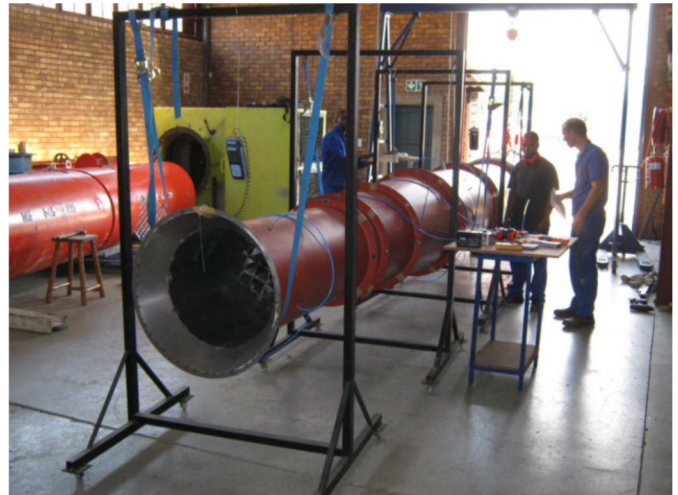
Figure 3. BS848 fan test duct
