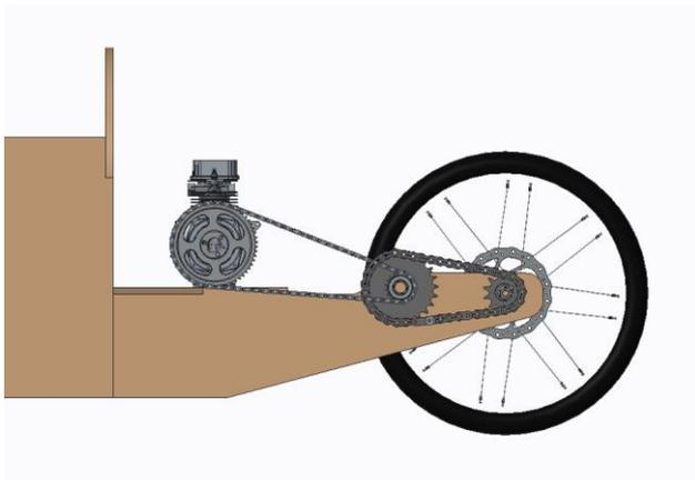
Fig. 3. Internal combustion engine chain drive propulsion system.
