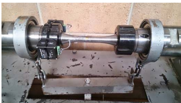
Figure 4 - Strain logging configuration
