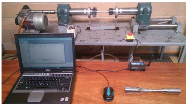
Figure 3 - Rotating bending fatigue testing machine
