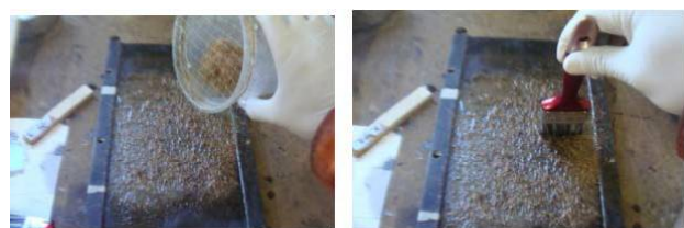
Figure 2 - Hand lay-up a) fibre distribution and b) resin distribution
