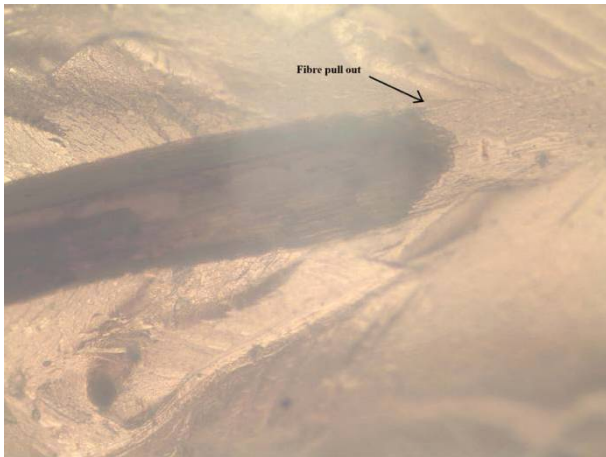
Figure 7 - Sample fractured specimen showing fiber pull out feature
