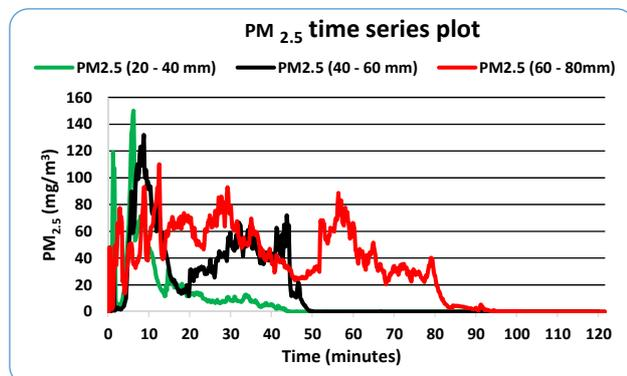
Figure 2: PM<sub>2.5</sub> time series plots for the three coal particle sizes in a high ventilation stove
