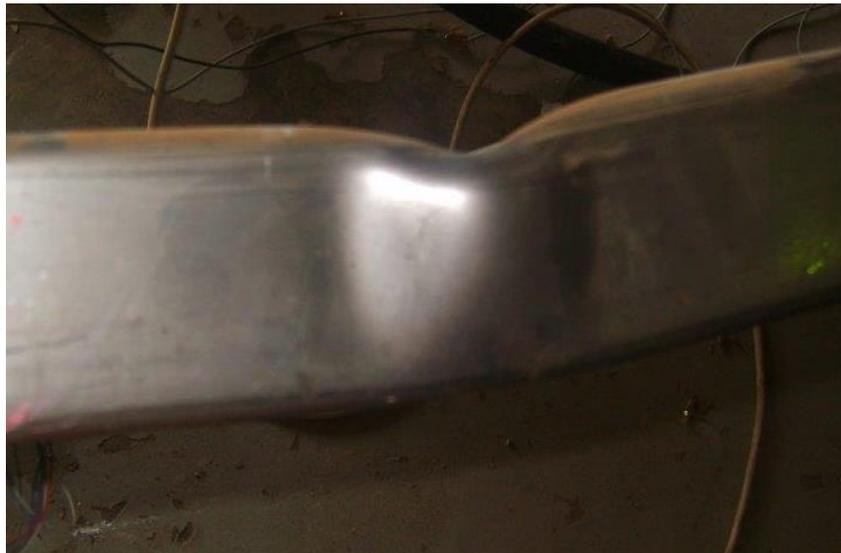
Figure 11 Inward distortional buckling
