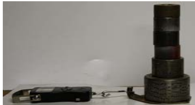
Figure 6. Test set-up to establish the coefficient of friction.
