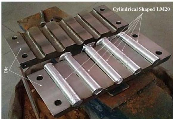
Figure 2. LM20 cylindrical shaped specimens
