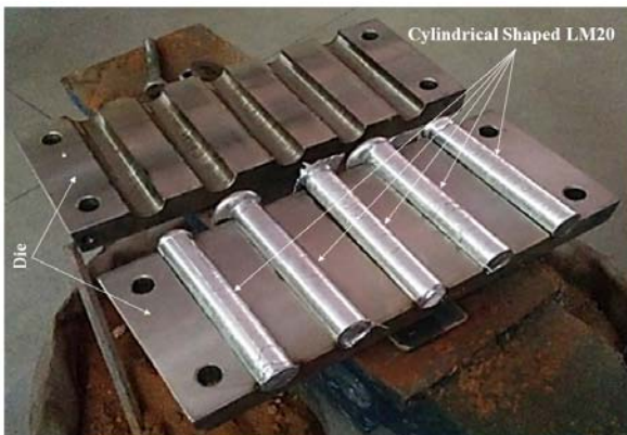
Figure 2. LM20 cylindrical shaped specimens
