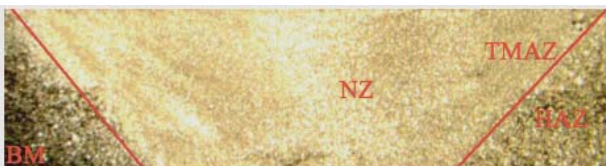
Fig. 5: Macrostructure of the welded joint
