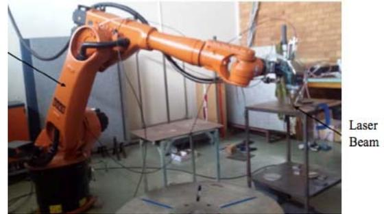
Fig. 2: Experimental setup of Kuka robot and laser beam
