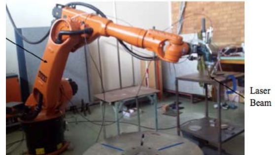
Fig. 2: Experimental setup of Kuka robot and laser beam
