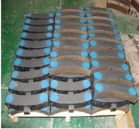
Fig. 1: The new low friction brake blocks being used from a wagon company to replace cast iron brake shoes [14]
