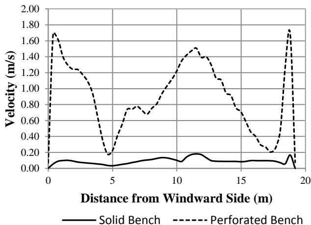
FIGURE 17: VELOCITY DISTRIBUTION COMPARISON AT 5M
