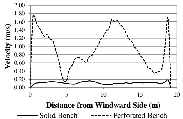
FIGURE 19: VELOCITY DISTRIBUTION COMPARISON AT 15M
