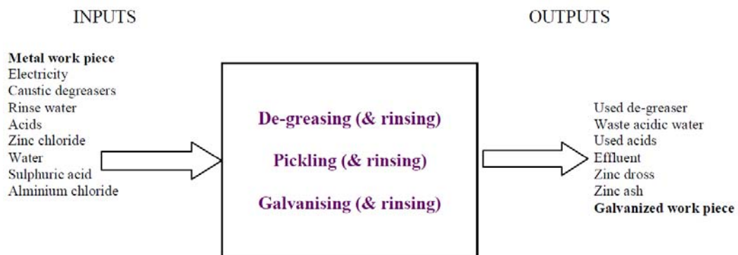
Fig.3. Galvanizing process flow chart
