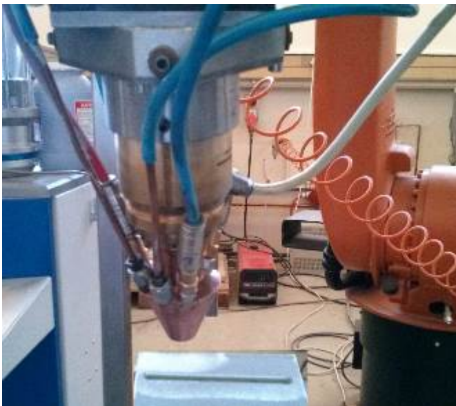
Fig. 1. Experimental setup of the LMD system
