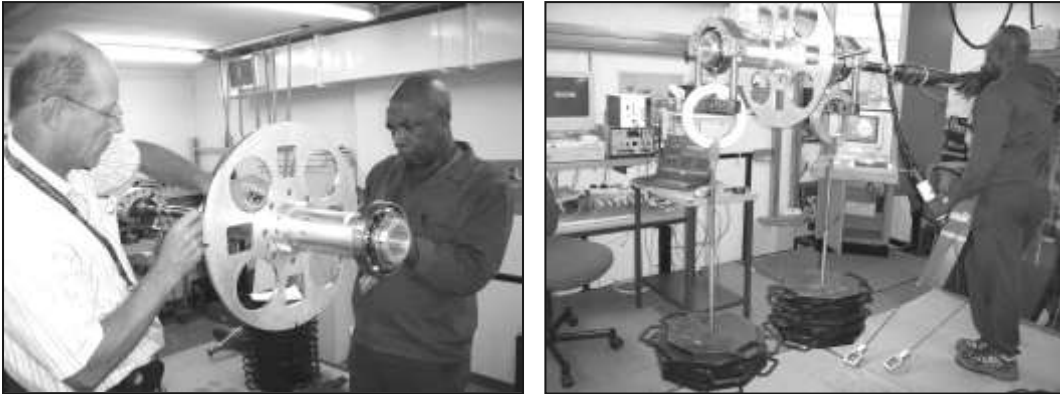
Figure 15. Calibration body fitted to the four-component optical fibre balance.
