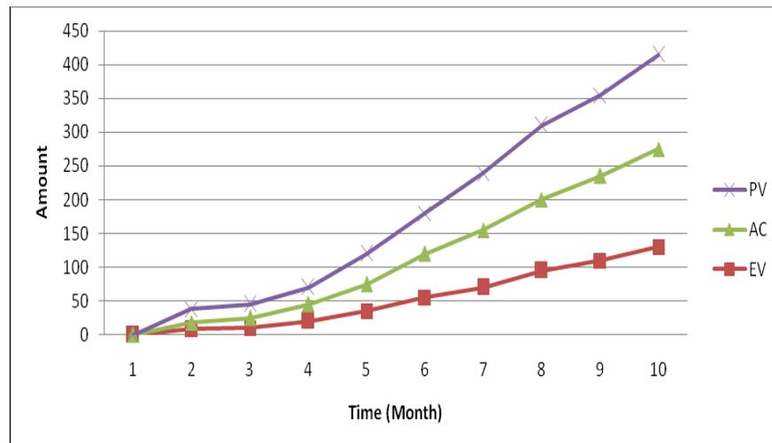
Figure 4: An Illustration of PV, EV and AC
