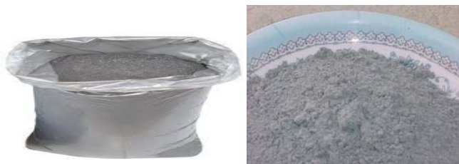
Fig. 3 Amorphous RHA from incineration and finely ground
