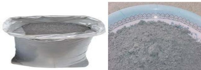
Fig. 3 Amorphous RHA from incineration and finely ground
